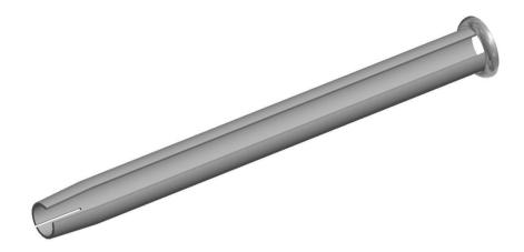
The Domed Friction Lok is designed to be easily installed in poor ground conditions, providing maximum load capacity across a wider range of installation angles. The uniquely designed and tested domed ring reduces point loading and resultant premature peeling.
