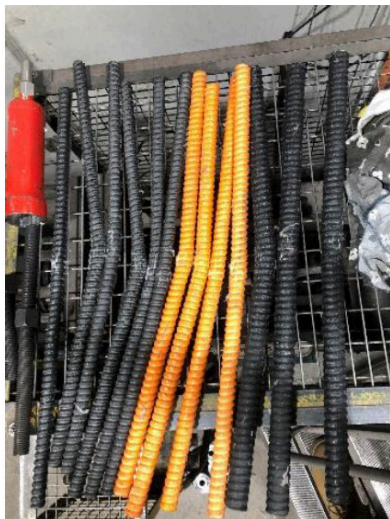
Samples after flexural test: 22, 25 and 32 mm dowels (left to right)
