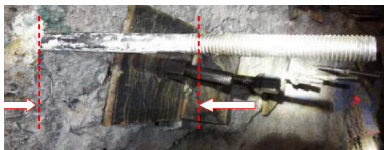
Yield-Lok displacement in full resin column grouted encapsulation
