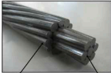
Grade composite cable showing High Tensile and Mild Steel wires
