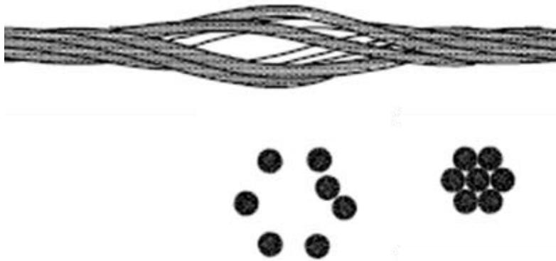
**FIG 4** – ...Typical Cable Bolt (Hutchinson and Diederichs, 1996).
