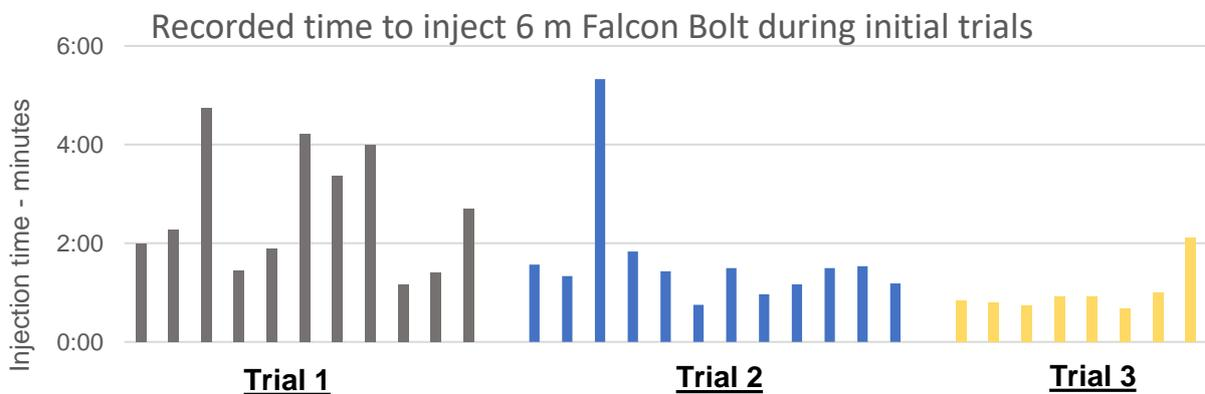
**FIG 9 – Injection time per bolt.**
