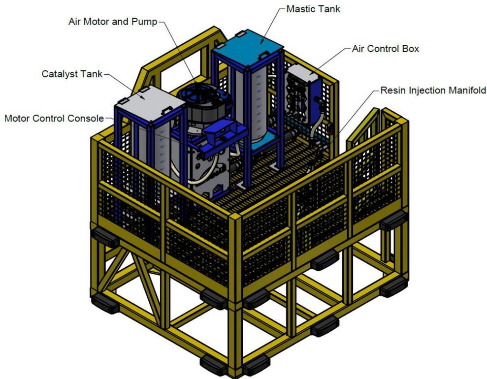
**FIG 8 – Resin injection IT basket.**
