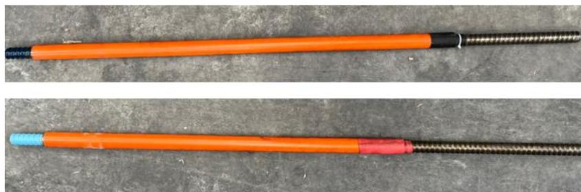
**FIG 6** – Bolt configuration for embedment length testing.
