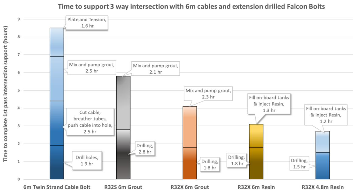
**FIG 7** – ‘Time on Bolt’, Installation steps and times for 6.0 m twin strand cable bolt and various Falcon Bolt configurations.
