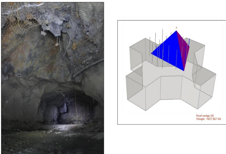
**FIG 1** – (Left) intersection wedge failure leading to abandonment of development and bypass development. (Right) Typical kinematic wedge assessment to aid ground support design or failure back analysis.
