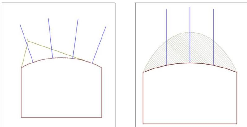
**FIG 3** – (Left) Kinematic wedge analysis, (right) parabolic arch method.
