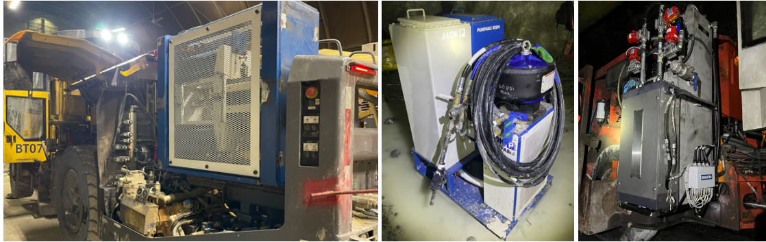
Figure 6 On-board high-pressure bulk transfer pumps. Shown are high-volume, multiple-shot mobile air-operated skid and single-shot pump options
