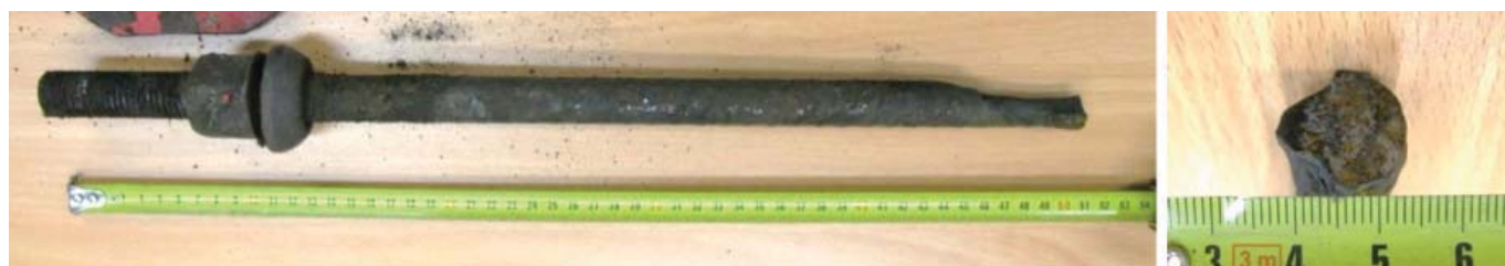
FIG 4 – Mine 3: bolt broken at 15 t during load test.
