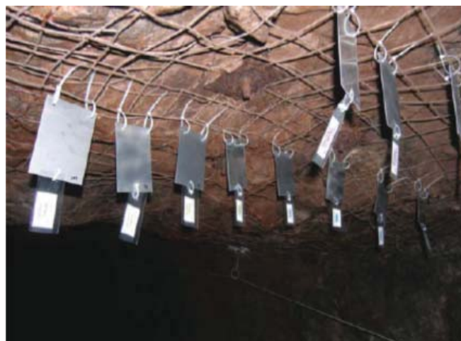
FIG 5 – ASTM Standard G4 coupons (Dorion, Hadjigeorgiou and Ghali, 2009).
