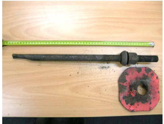
Figure 4. Severe localized pitting corrosion on load tested bolt.
