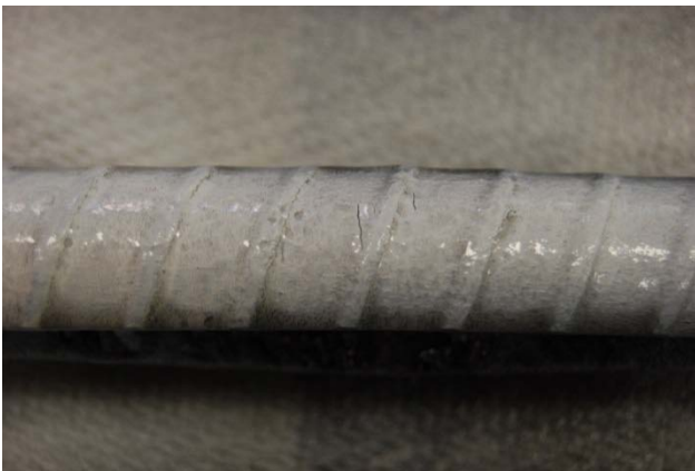
Figure 9b. Magnetic particle inspection revealing a crack.
