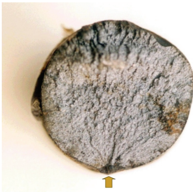
FIG 1 - View showing evidence of brittle failure of a rock bolt (Crosky et al , 2002).
