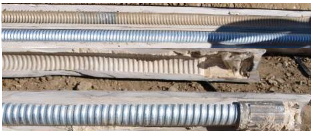
Figure 11 Resin mixing results from testing completed (a) One example of the resin mixing completed using the paddle mixing device (b) One example of the resin mixing completed using the resin shredder mixing
