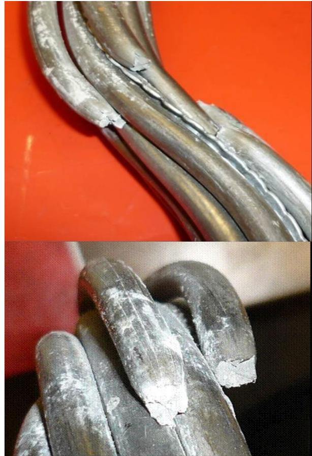
Figure 9. Cone and Cup strand failures.
