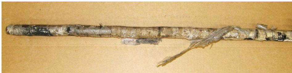
(a) 1 x 28 mm Pinched Ear, site 2:1 water based resin - extensive gloving with plastic film intact along 900 mm of bolt
