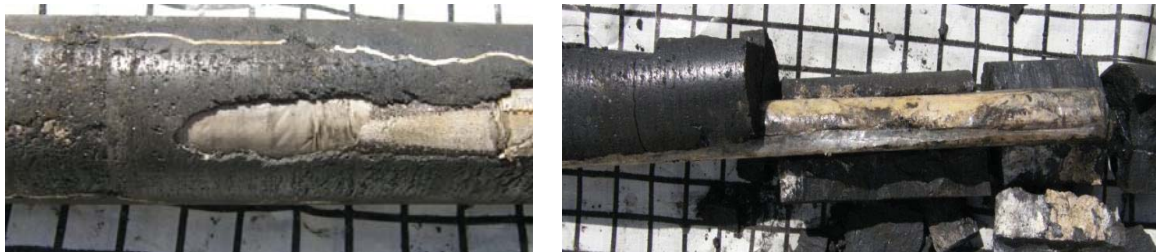
Figure 1 - 1 st site over-core: standard bolt, standard viscosity 2:1 water based catalyst resin
