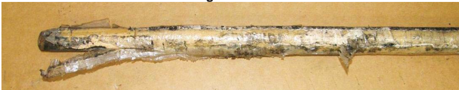
(b) Standard bolt, site 2:1 water based resin - extensive gloving with plastic film intact along 600 mm of bolt
