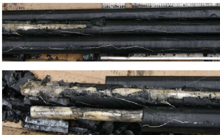
Figure 4 - Three over-cored bolts, 93:7 ratio mastic: catalyst oil based, standard viscosity
