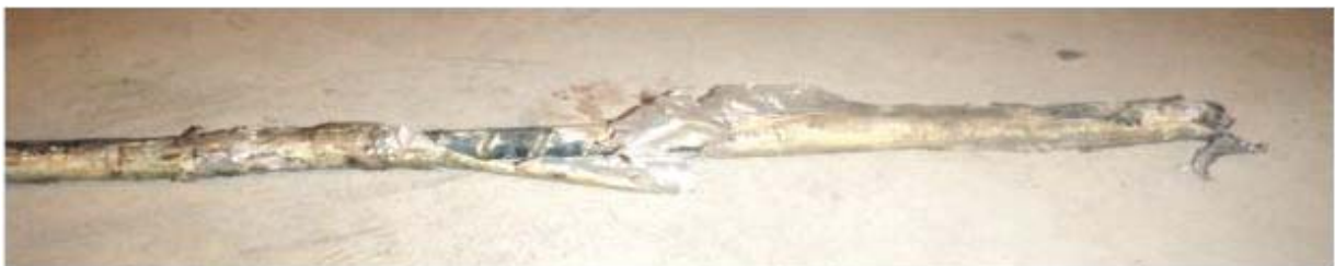
Figure 2 - Overcored bolt taken from the support pattern
