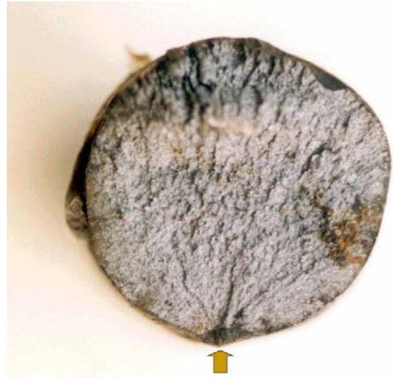
Fig. 1. View showing evidence of brittle failure of a rockbolt [1].
