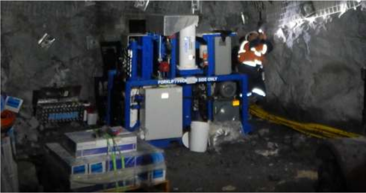
Figure 3 J-Lok P Installation onto Boltec drill. Resin and catalyst load cylinders are mounted on the side of the Boltec and injection cylinders and 100 litre accumulators are mounted on the top of the Boltec. A J-Lok P Skid Mounted resin injection system being utilised for cable bolting applications and connected to 1000V Jumbo starter power supply
