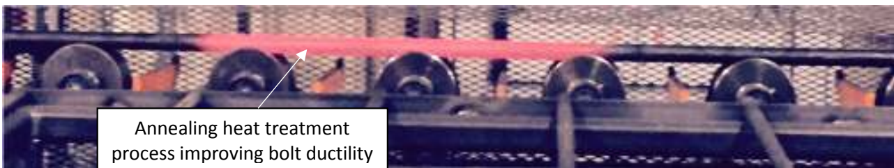
Figure 9 Annealing of the MPA bolt and finished bolts strapped after manufacturing
