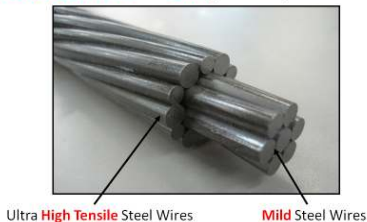
Figure 11 The GRACOM cable showing both Ultra-High and Ultra-Low grade composite strand construction
