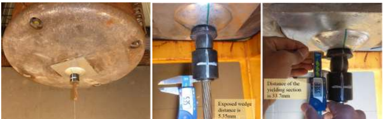
Figure 13 Post testing SECTA cable with Barrel and Wedge and prior test GRACOM Cable with Yield Tube and Barrel and Wedge arrangement, (De Zoysa et al, WASM)
