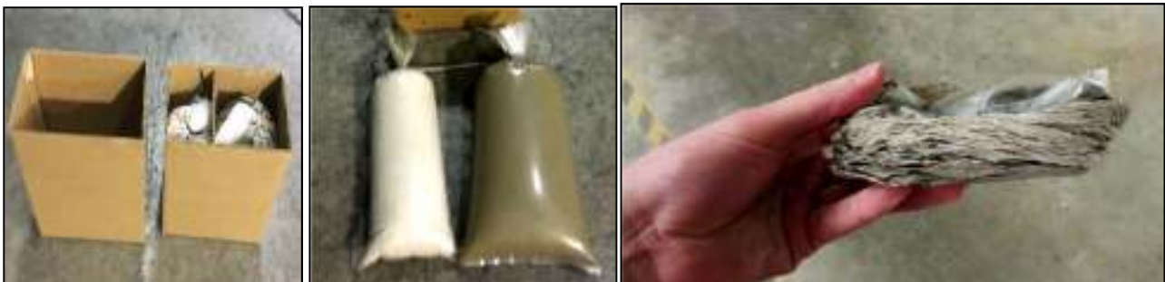
Figure 5 Resin shown in 2:1 catalyst/resin mix ratio and bag shown after resin injection. 18kg resin/catalyst are in each 600 mm long boxes, easy transported to varying locations for use
