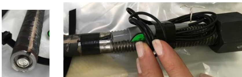
Figure 3: Pictures of rockbolt and pressure cell setup: a) pressure cell countersunk in head of bolt and b) wiring at foot of bolt for attachment to logger
