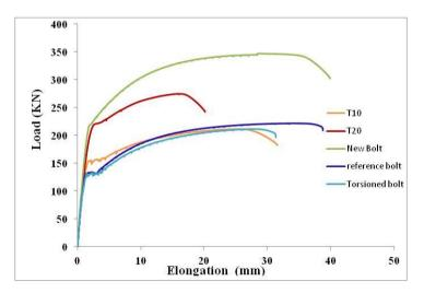
Figure 6 - Load displacement profiles of various bolts
