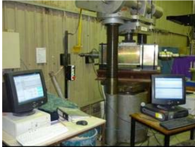
Figure 3 - Assembled double shear apparatus in 500 tonne testing machine
