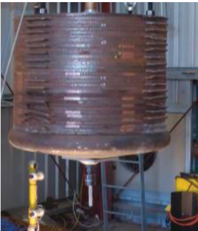
17.8mm Single Yield Tube before dynamic testing
