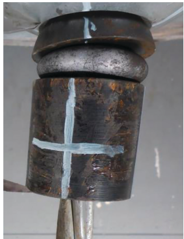
17.8mm Single Yield Tube after dynamic testing. Yield tube increased energy dissipation by 10kJ
