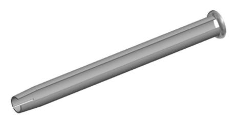
The Domed Friction Lok is designed to be easily installed in poor ground conditions, providing maximum load capacity across a wider range of installation angles. The uniquely designed and tested domed ring reduces point loading and resultant premature peeling.
