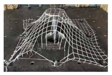
SpiderWeb Mesh is a high strength polyester geofabric designed for reduced manual handling and easy installation with existing mining equipment. The module conforms well to rock undulation and provides alternative support to welded steel mesh in extreme mining conditions.
